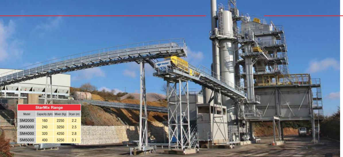
The StarMix range incorporates as standard 4, 5 or 6 hot stone storage compartments above the mixer which can be increased to 13 by installing a modular diverter section beneath the screen.
