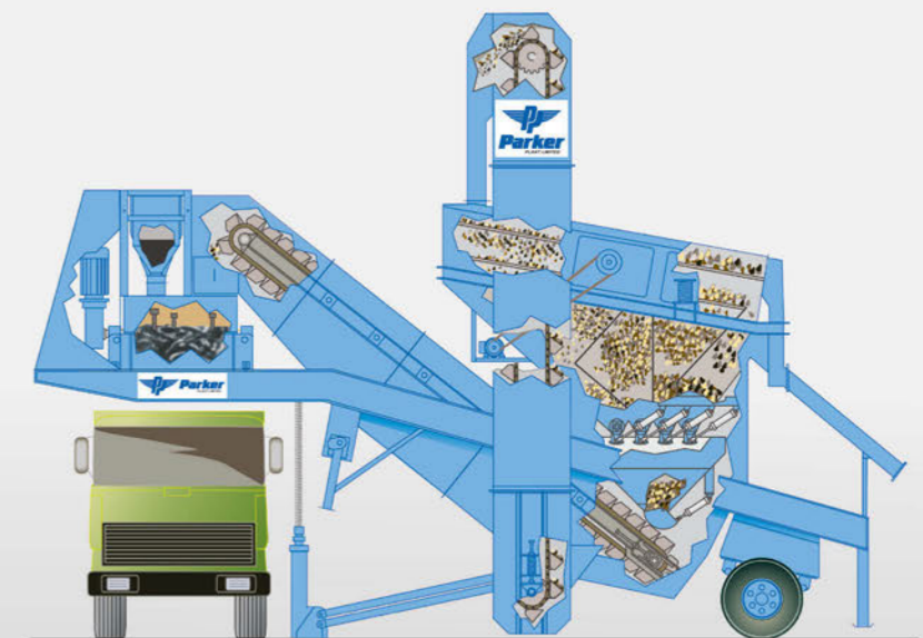
Material flow for a RoadStar 1500.
