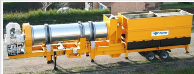
Mobile cold feed unit, dryer and burner
