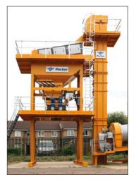
Quick erect, modular tower; heavy duty aggregate screen with-in a fully sealed dust housing; access stairways and platforms for maintenance at all levels; load-cell mounted batch weigh hoppers for aggregate, bitumen & filler. Twin shaft, direct gear/motor drive high efficiency paddle mixer, hard wearing replaceable abrasive resistant liner plates, paddle arms and tips. Discharge to truck or mixed material storage facility.
