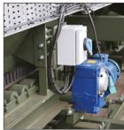
Compact, robust, modular cold feed unit with a choice of number and configuration of hoppers with high accurate AC variable speed inverter controlled direct drive motor/ gear units.
