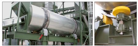
Easily transported aggregate dryer with advanced design of internal lifters optimising thermal efficiency for maximum heat transfer. Choice of multi-fuel burners. Nylon support & thrust rollers reduce wear, vibration and noise.
