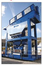
Quick erect, modular tower; heavy duty aggregate screen with-in a fully sealed dust housing; access stairways and platforms for maintenance at all levels; load-cell mounted batch weigh hoppers for aggregate, bitumen & filler. Twin shaft, direct gear/motor drive high efficiency paddle mixer, hard wearing replaceable abrasive resistant liner plates, paddle arms and tips. Discharge to truck or mixed material storage facility.
