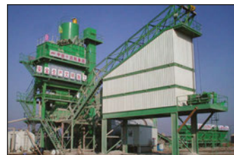
210 tonne mixed material storage - China
