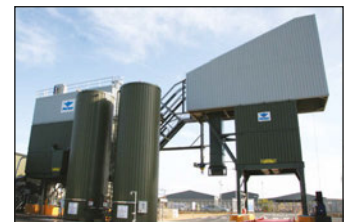
Parallel 200 tonne, 4 silo, mixed material storage system - UK
