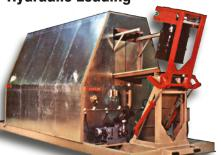
Drums up to 200 litres in size with tops removed are secured to trolleys by drive pin method, they are then rolled on to the fork for inverting on to the gravity track
