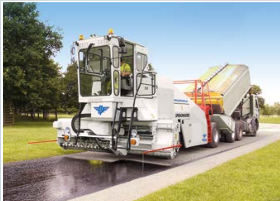
Chip spreading in operation with chipping supply truck on tow.
