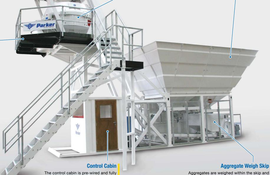
tested prior to despatch and forms part of the main structure. The Constar PLC based control system gives fast, accurate measurement of mix ingredients, as well as monitoring dynamic aspects of the plant for continuous and safe operation. **Aggregate Weigh Skip**
