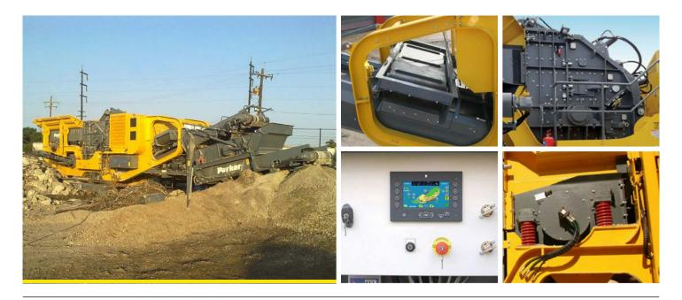
The HS1112R is a track mounted mobile crusher utilising the aggressive Parker 1112 horizontal shaft Impactor designed for processing a wide variety of materials including demolition and recycling applications.
