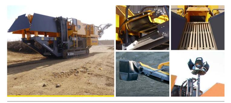
The compact JR0960 is ideal for primary crushing in quarrying operations or for demolition contractors where setup speed and operating space is restricted.
